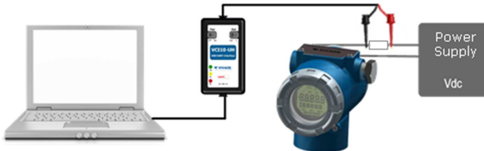
Figure 3.5 – Transmitter installation for configuration with external power supply and 250 ohms resistance.
