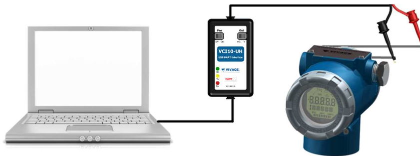
Figure 3.6 – Transmitter installation for configuration using VCI10-UH to power the device.
