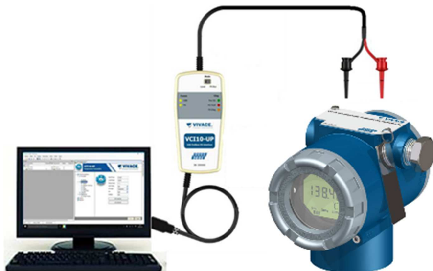
Figure 3.5 – Configuration diagram of VTT10-FP with VCI10-UP.
