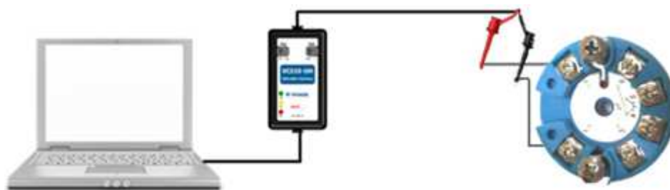
Figure 3.2 – Transmitter installation for configuration using VCI10-UH to power the device.
