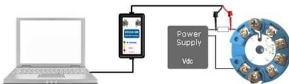
Figure 3.1 – Transmitter installation for configuration with external power supply and 250 ohms resistance.
