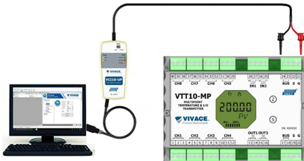
Figure 3.5 – Configuration diagram of VTT10-MP with VCI10-UP.
