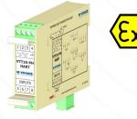
VTT10-P is a temperature transmitter for DIN rail mounting, that accepts TC, RTD, Ohm and mV sensors, generating 4-20 mA current signal (HART® 7 model) or a digital signal (Profibus-PA model), according to the measurement type and user configuration. The HART®/4-20 mA model has two open-collector outputs for alarms or on/off signals.
