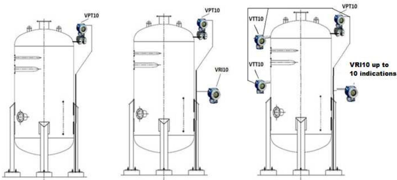
In some situations, the Profibus-PA device is installed in a location that is inaccessible to the operator. In these cases, the Remote Indicator VRI10-P makes it easy to see the monitored variable by the operator. He can have up to 10 indications of various device in the Profibus-PA network.
