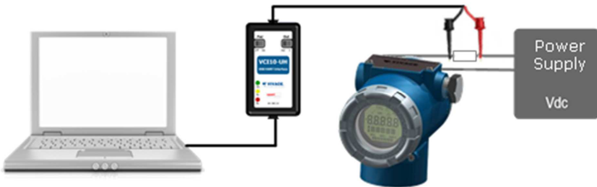
Figure 2.1 - Interface configured to not power device.
