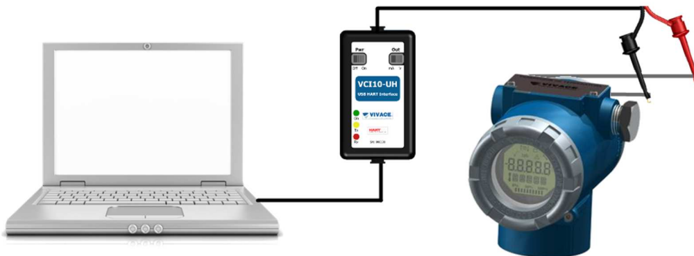
Figure 2.2 - Interface configuration to power device.
