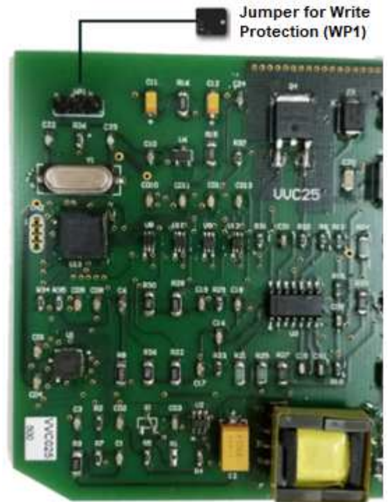
Figure 3.1 – Hardware write protection.
