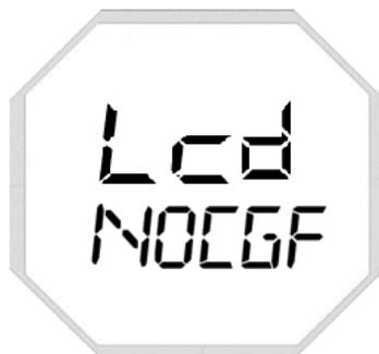
Figure 3.7 – LCD indication of No LCD Configuration.
