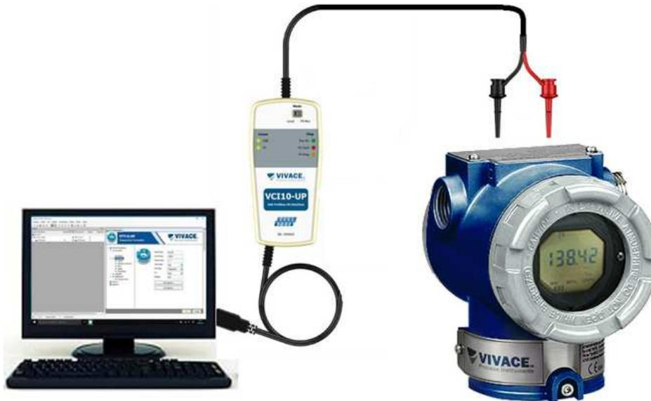
Figure 3.5 – VRI10-P configuration diagram with VCI10-UP
