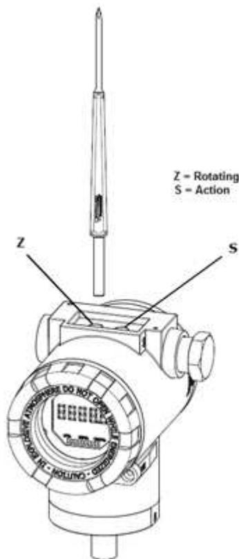
Figure 3.1 – Z and S orifices and magnetic screwdriver.
