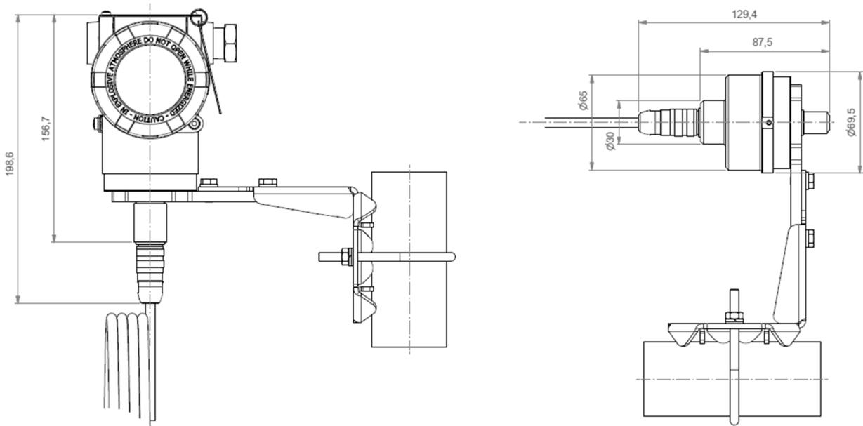
Figure 2.13 – Remote sensor dimensional drawing.
