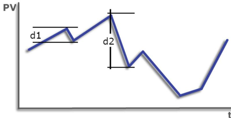
Figure 3.12 – Example of reversal occurrence on VTP10-H.
