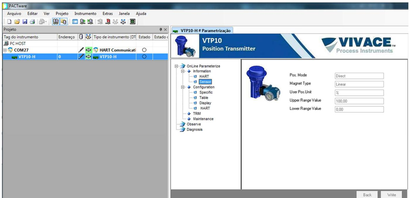
Figure 3.13 – DTM sensor configuration screen for VTP10-H.
