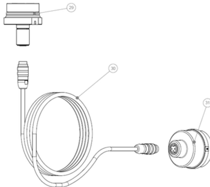
Figure 4.2 – Exploded view for VTP10-H remote sensor.
