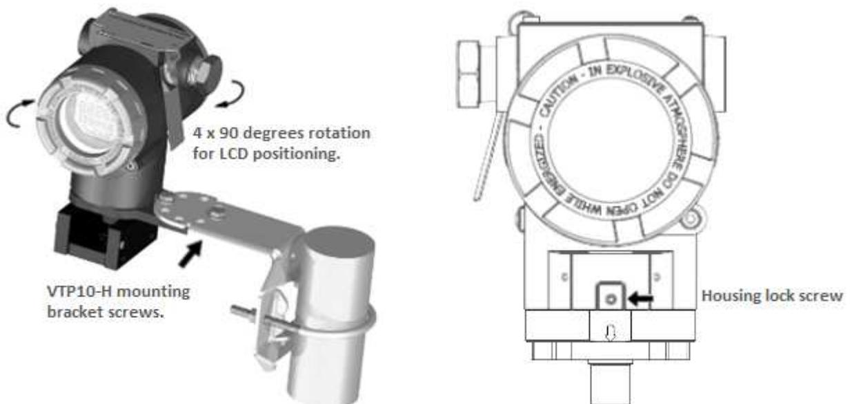
Figure 2.3 – VTP10-H bracket fixation and housing 4 x 90° rotation.
