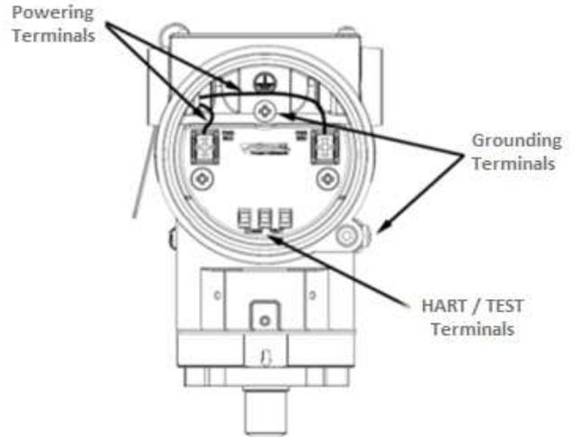
Figure 2.9 – VTP10-H connections and terminal description.
