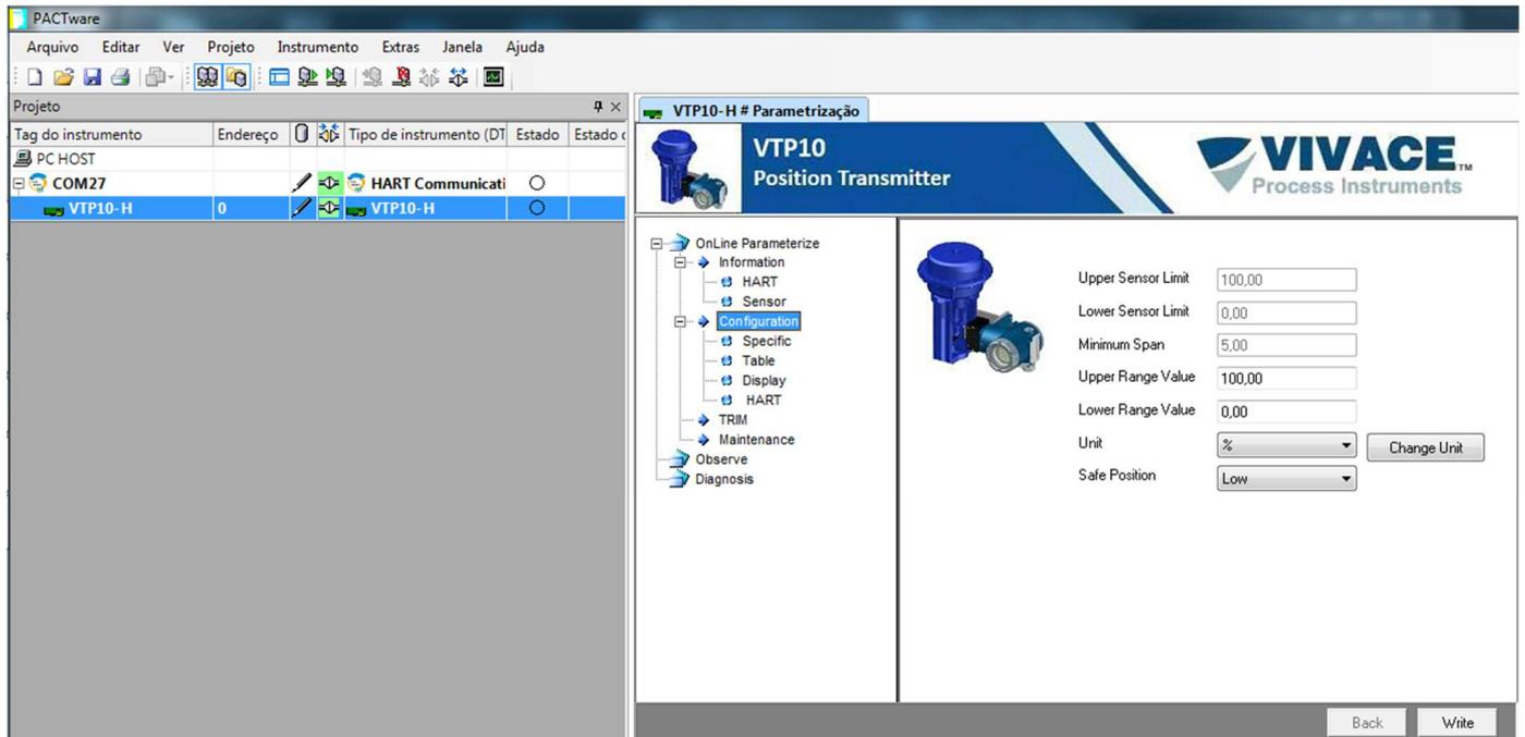
Figure 3.12 – DTM work range configuration screen for VTP10-H.
