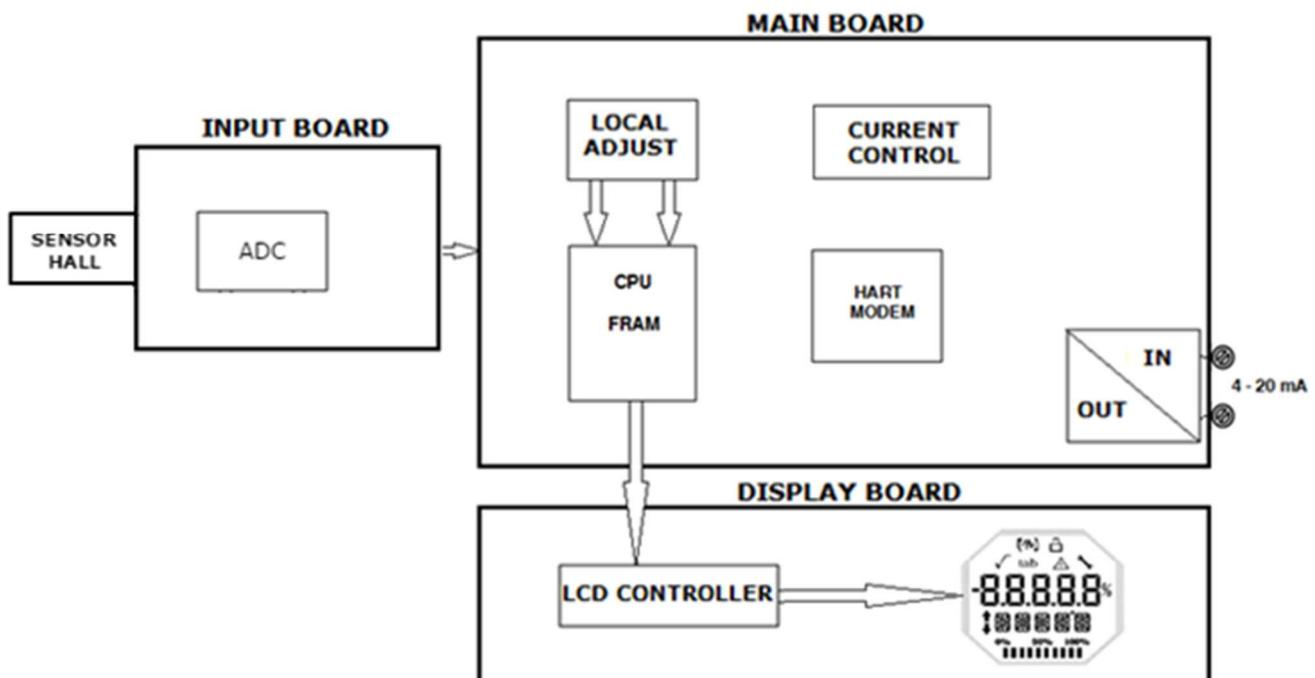
Figure 1.1 - VTP10-H block diagram.
