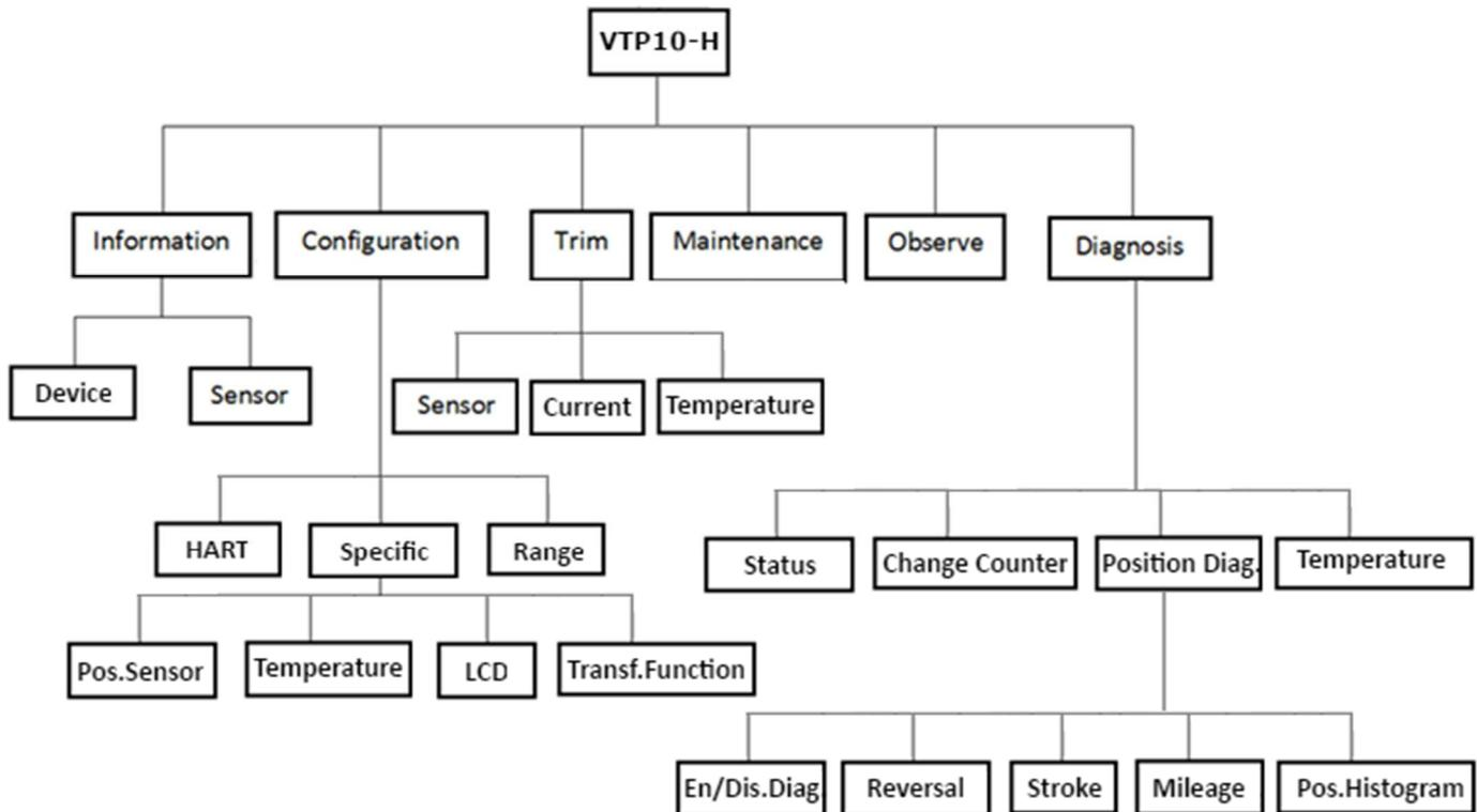
Figure 3.9 – VTP10-H programming tree.
