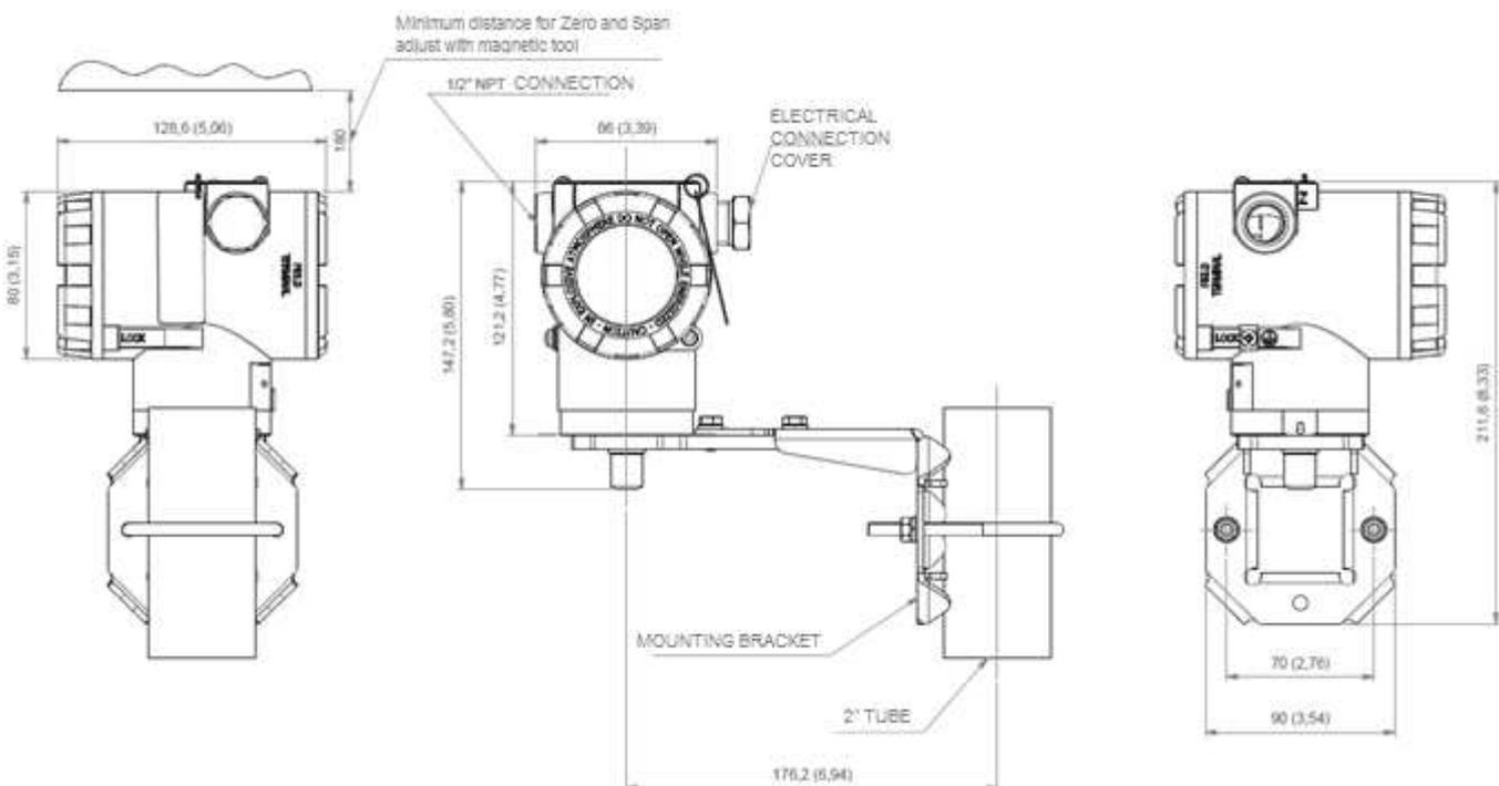
Figure 2.1 – Dimensional and mounting drawings for VTP10-H.
