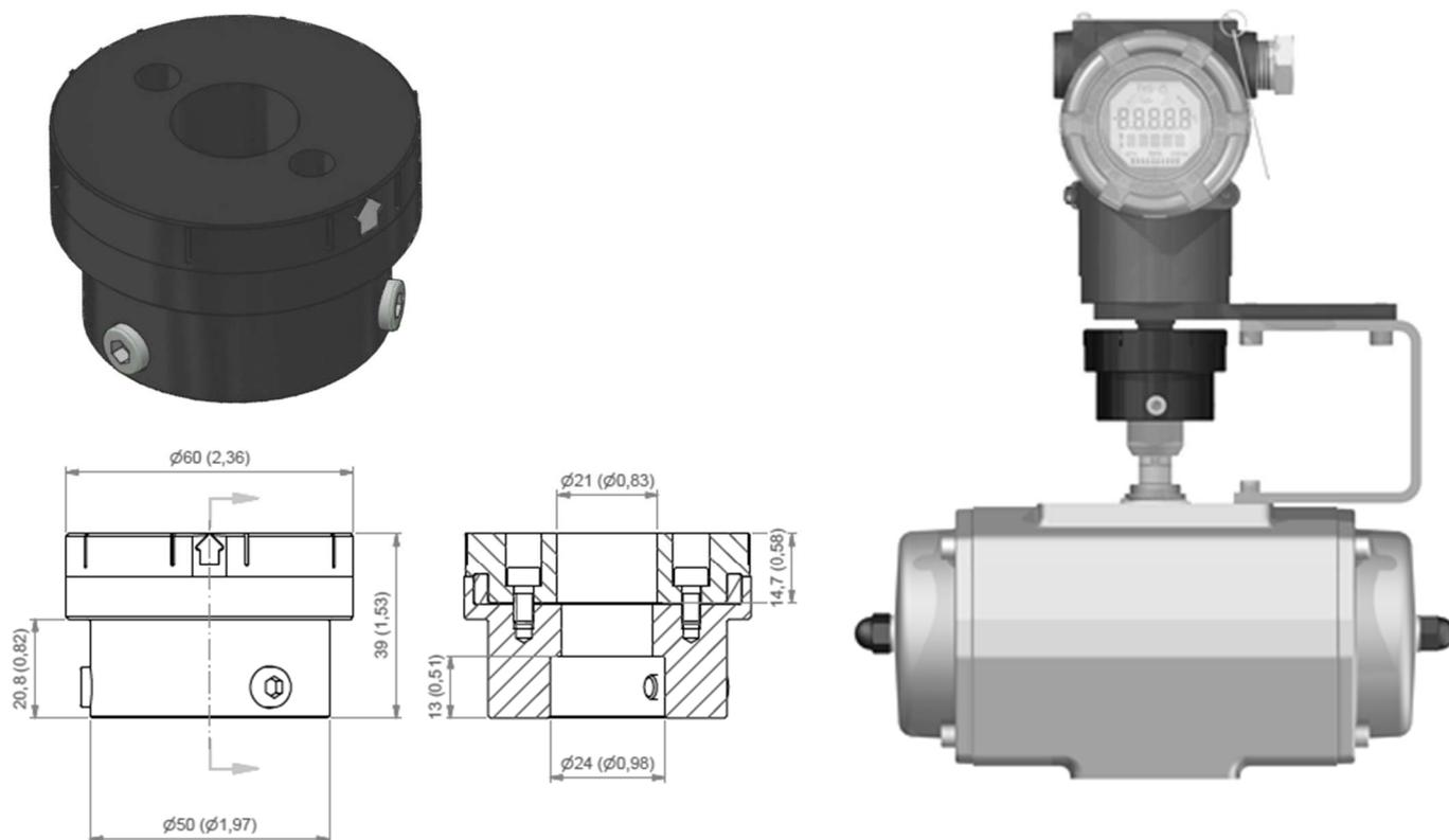
Figure 2.11 – Dimension and assembly of rotative magnet.
