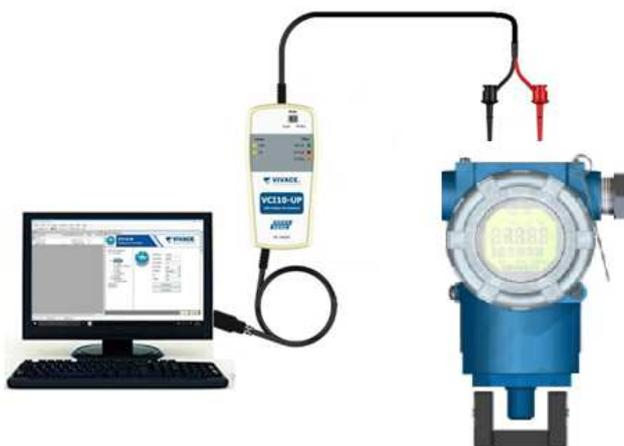
Figure 3.5 – VTP10-P configuration diagram with VCI10-UP.
