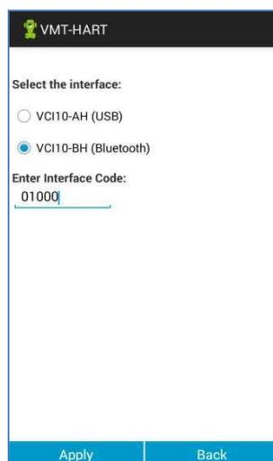
When using VCI10-BH (Bluetooth), user will need to enter the interface code for Bluetooth (located on the back of battery cover). This code also can be found on the device list identified for Bluetooth connection. The Bluetooth identification name for VCI10-BH is composed by “BH-” + Interface Code.
