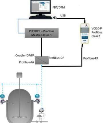
VCI10-UP is able to work with or without the main network controller. This is only possible thanks to the powerful processor inside VCI10-UP which acts as secondary master (Master Class2). VCI10-UP can be set in mono or multi-master PROFIBUS operation mode.
