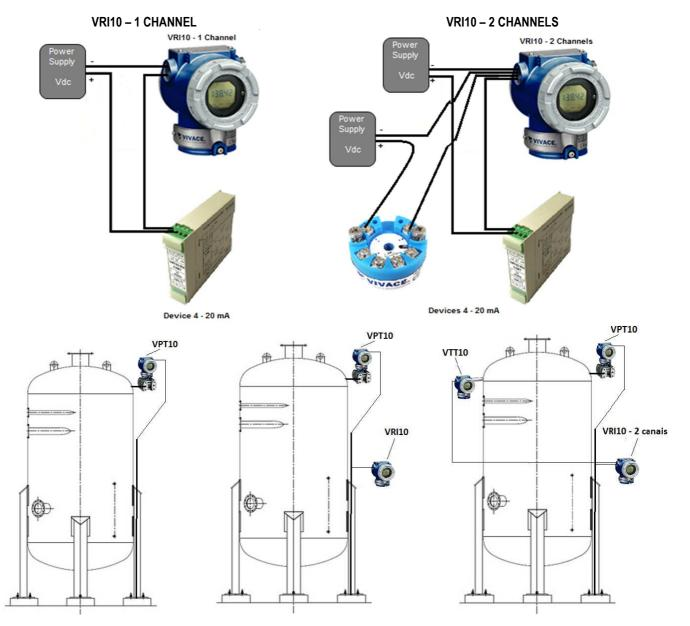
In some cases the place where a 4 - 20 mA device is installed is inaccessible or difficult to be reached by the operator. In this case VRI10-I Remote Indicator facilitates monitored variable visualization.
