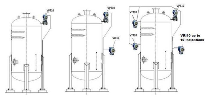
In some situations, the Profibus-PA device is installed in a location that is inaccessible to the operator. In these cases, the Remote Indicator VRI10-P makes it easy to see the monitored variable by the operator. He can have up to 10 indications of various device in the Profibus-PA network.
