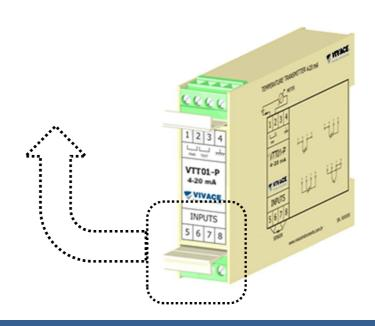
RTD – Temperature sensor based on resistance with 2, 3 or 4 wires connection
