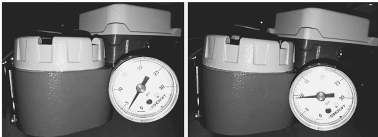
Figure 3.3 – Pilot pressures for CWR 0% and 100%, respectively.
