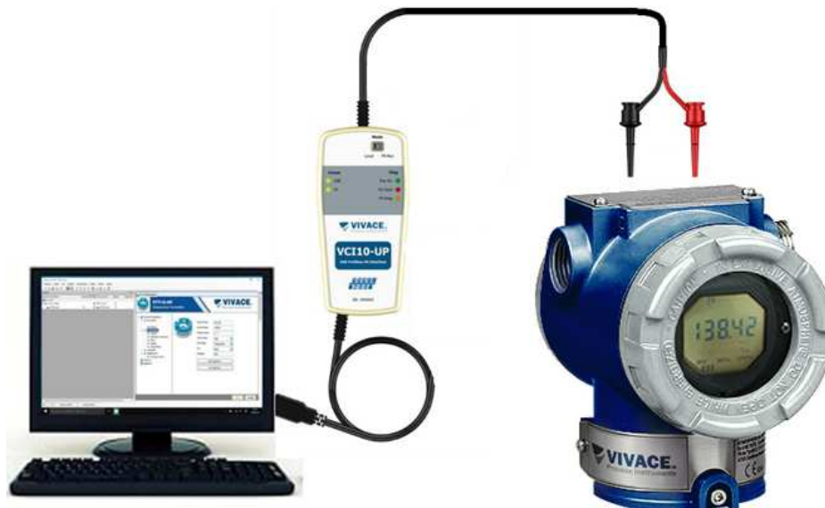
Figure 3.5 – Configuration diagram of VAP10 with VCI10-UP.
