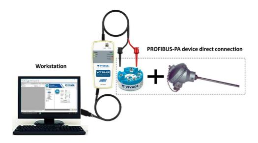
Figure 4.2: Connection schematic when using the operating mode "Local".
