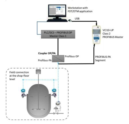
Figure 4.4: Schematic of VCI10-UP installation in parallel to a PROFIBUS architecture.
