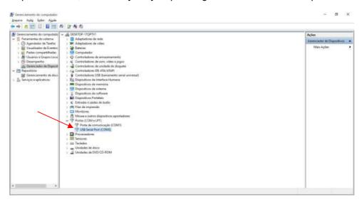
Figure 2.2: Automatic creation of the USB Serial Port.
