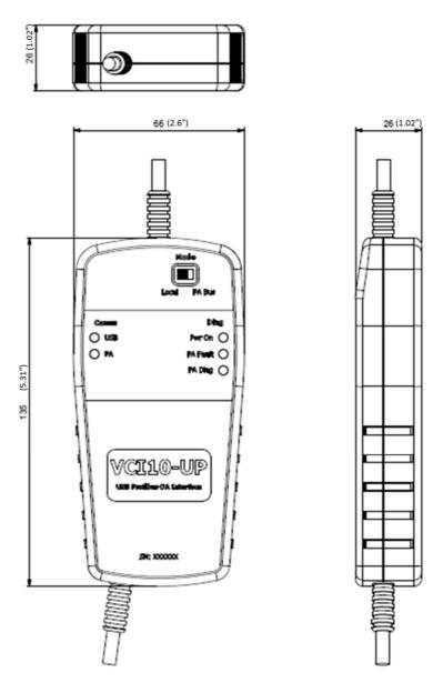
Figure 3.1: Mechanical Dimensions of VCI10-UP.
