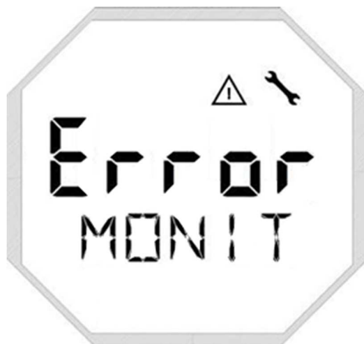
Figure 4.1 – Error indication on VHC10-F monitoring.
