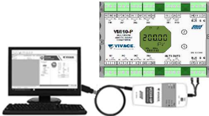
Figure 3.5 – Configuration diagram of VMI10-P with VCI10-UP.
