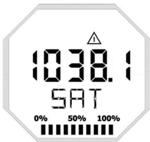
Figure 3.14 – Indication of measurement saturation on VPT10-H.
