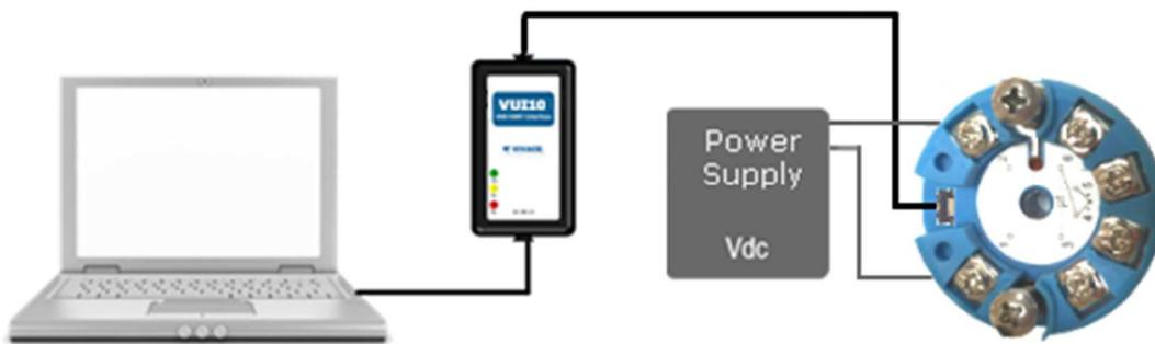
Figure 3.1 - Connecting VUI10 interface to VTT01-H with external power supply.
