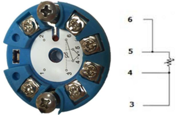
Figure 2.6 - RTD or resistive 3-wire connection.
