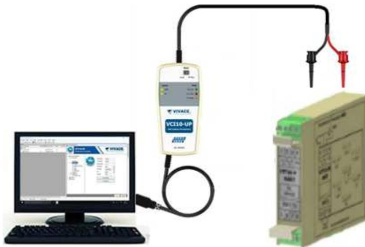
Figure 3.1 - Configuration diagram of VTT10-PP with VCI10-UP.
