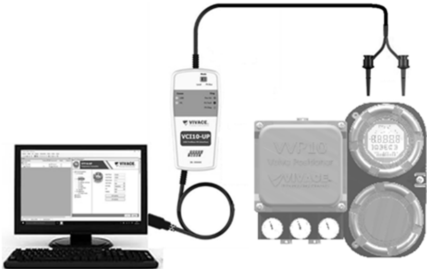
Figure 3.4 - Wiring diagram of VCI10-UP interface to VVP10-P.
